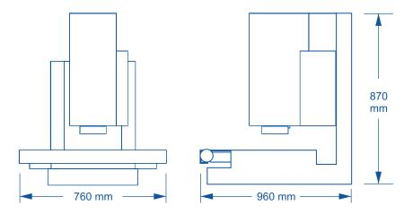
Machine Weight: 175 Kg Crated Weight: 300 Kg
