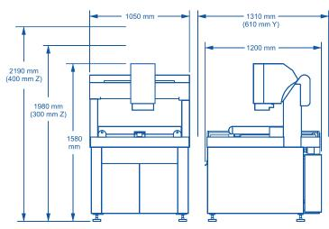
Machine Weight: 960 Kg Crated Weight: 1020 Kg
