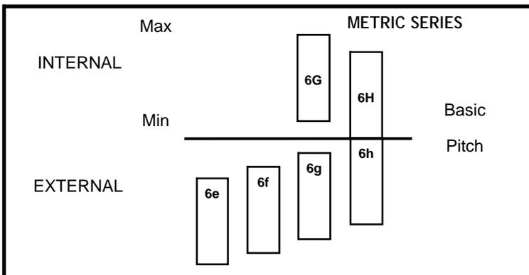
Here again we see a difference in the inch and metric systems. In the Unified, there is only one allowance available and it is only applied to the external thread. For metric, you can apply allowances to the internal also. In both the internal and external the 'h or H' signifies an allowance factor of zero. The 'G' is the only allowance for internal threads and the 'g' is the smallest allowance available for external, the 'f' being more, and the 'e' being the greatest allowance.
