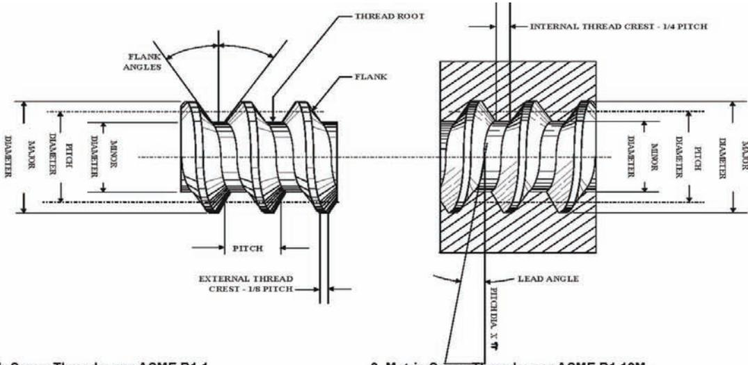
1. Unified Inch Screw Threads: per ASME B1.1
