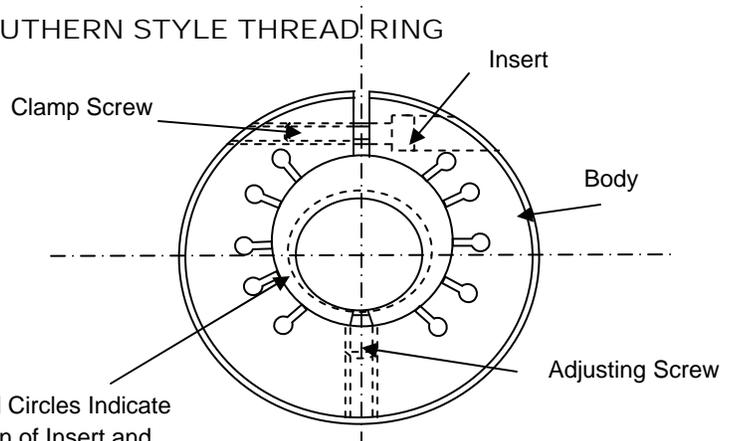
Etched Circles Indicate Position of Insert and Body For Re-Assembly.
