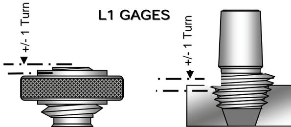
The L1 when screwed onto the pipe or plug into the hole "hand tight" should be flush with the end of the pipe or the hole, or gage plane, within 1 turn.
