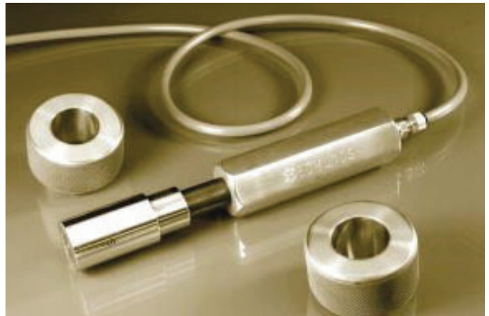
Two-nozzle air plug, with masters, for measuring an inside diameter
