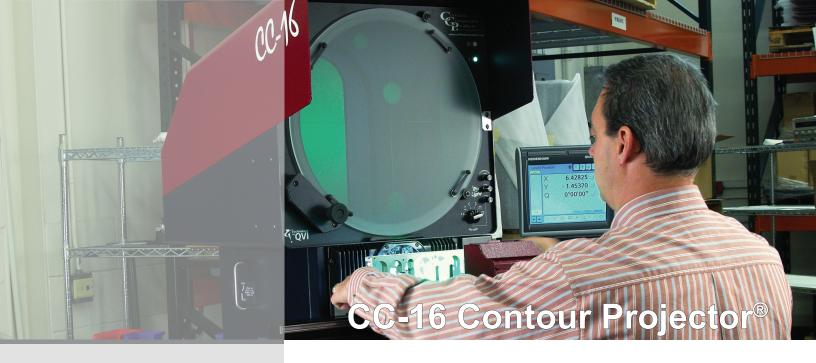
The CC-16 is a top quality optical comparator designed for high performance on the shop floor. The 16" diameter screen displays crisp, evenly illuminated images at every available magnification.
